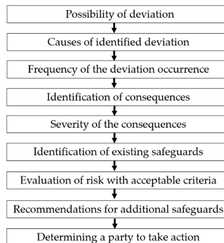
Figure 1. The steps used in hazard identification from derived deviations (adapted from [27]).
